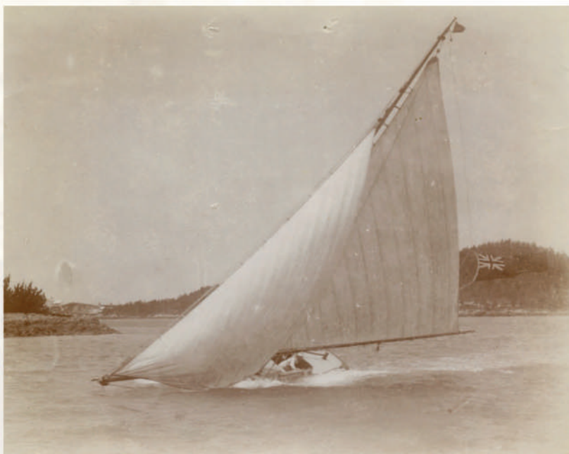
A small Bermuda sloop with the classic "Bermuda Rig" (fore and aft sails) used by most modern yachts and invented in Bermuda before 1674 (Photo taken about 1910).
