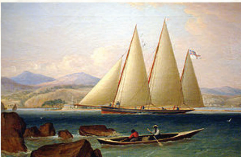
A large Bermuda sloop, built for the British Royal Navy, about 1750, with typical raked mast and fore-and-aft Bermuda Rig: the greatest invention in sailing technology after the European "Square Rigger": Dr. Edward Harris
