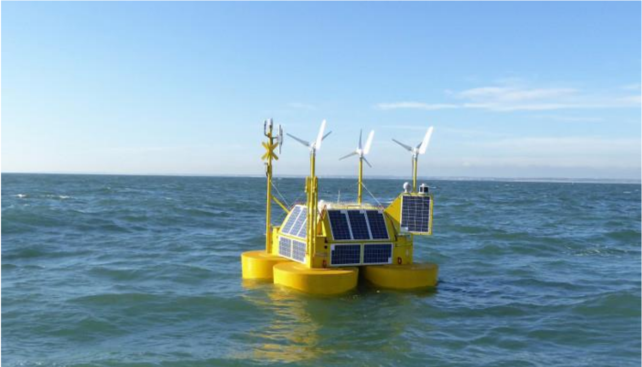
Figure 5 Example of a floating lidar device. (Image courtesy of EOLOS Floating Lidar Solutions)
