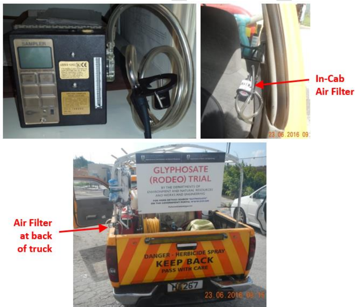
Figure 1. Photographs of the air sample collection pump, applicator truck with sign and air sampling filter cartridges set up in the vehicle cab and at the back of the truck.
