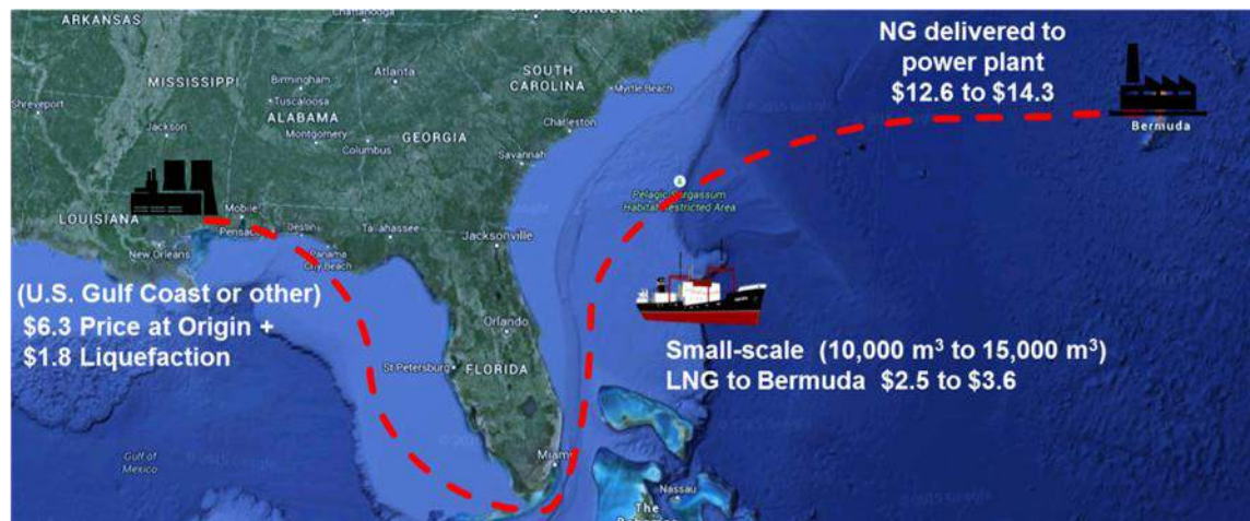
Figure 0.2: LNG Supply Chain to Bermuda (Cost per Million British thermal units)
