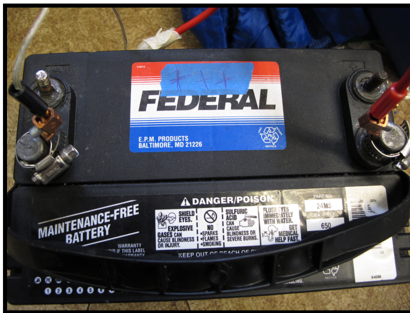
Figure 10: 12 volt car battery with hose clamp mounts to fit banana plugs at phase 2,3 and 4.
